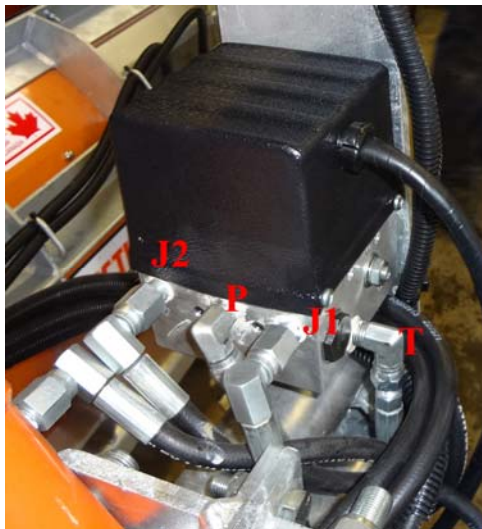
Manifold hose installation.
