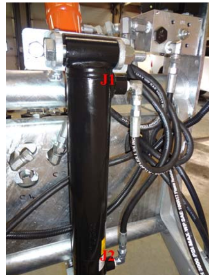
Jack hose installation 18".
