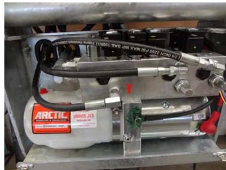
Wing plow power unit (P and T hoses installation 29")
