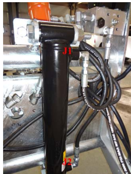
Jack hose installation 18".
