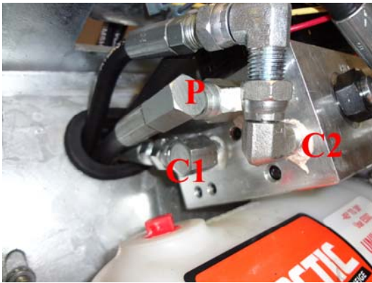
V plow power unit (P and T hoses installation)
